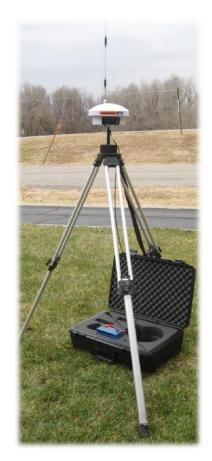
A solution where your machine is connected to a single base station which is moved or mounted permanently.
