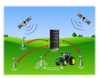
A "Network Solution" uses a group of bases to increase reliability and accuracy.
